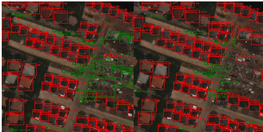
(c) Results of Faster R-CNN, ground truth on the left, predictions on the right
