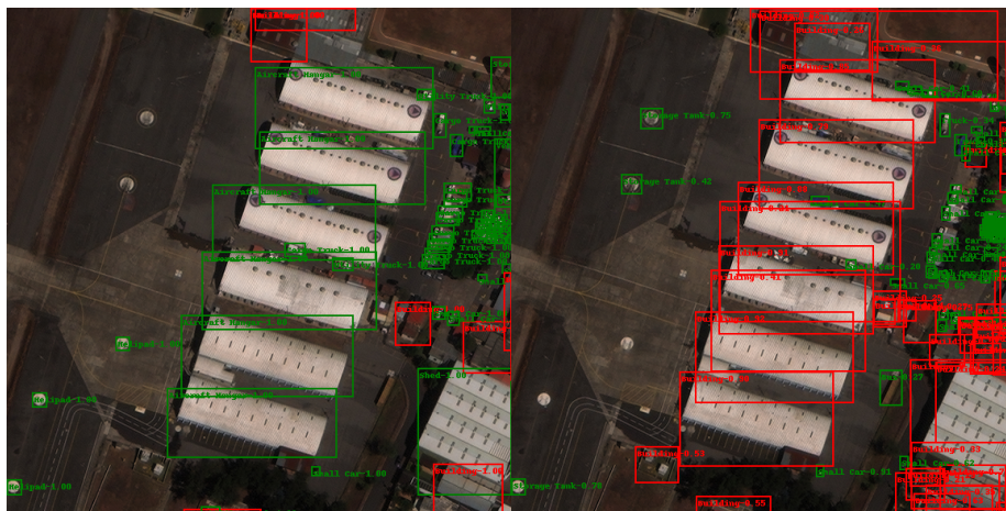
(a) Results of Faster R-CNN, ground truth on the left, predictions on the right
